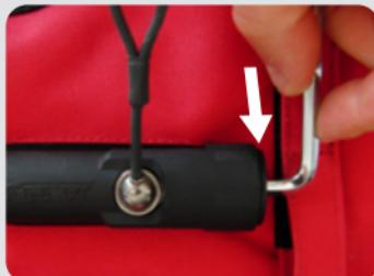
Finish screwing the bearing cap with the Allen key while still holding the key-ball. The bearing cap must be in contact with the cylinder. Do not overtighten or damage the parts.
