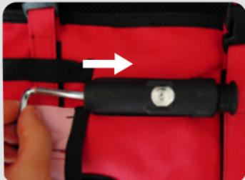
Replace the piston by using the Allen key or your finger. Make sure that the notch of the piston is in front of the hole where the key-ball is placed.
