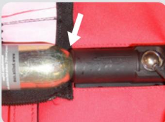
Lastly, insert a new CO<sub>2</sub> cartridge and screw it in completely without force. Make sure that the cartridge is sufficiently tight or is not screwed sideways. If your cartridge does not screw in easily without significant force it is possible that you have 'cross threaded' during insertion. In this case, unscrew the cartridge and start the process again until your cartridge goes in easily.
