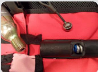
Following activation of the mechanical system (inflation of the airbag), the key-ball has been ejected and the spring is visible. Unscrew the empty CO<sub>2</sub> cartridge and remove it.
