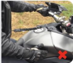
The fixing point resists over 150 kg. For example, do not use a plastic part. The fixing point is not in contact with any hot or sharp part of the motorcycle.
