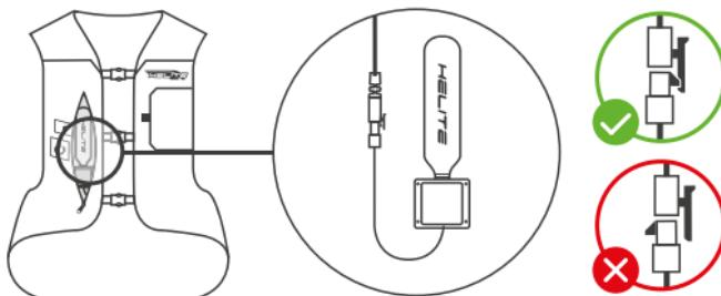
Check that the cartridge is connected to the CDU electronic card. Open the pocket on the right side of the airbag vest. Check the connection: connector in the right direction and locked. Close the pocket.
