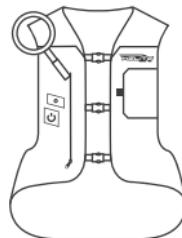
**2 Remove the empty cartridge.** To access it, open the pocket located on the right side of the airbag vest. Unplug the cartridge
