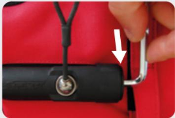
Finish screwing the bearing cap with the Allen key while still holding the key-ball. The bearing cap must be in contact with the cylinder. Do not overtighten or damage the parts.
