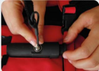
Replace the ball in its location. The ring around the ball should be positioned flat. Start screwing the bearing cap by hand while holding the key-ball firmly.
