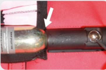
Lastly, insert a new CO2 cartridge and screw it in completely without force. Make sure that the cartridge is sufficiently tight or is not screwed sideways.
