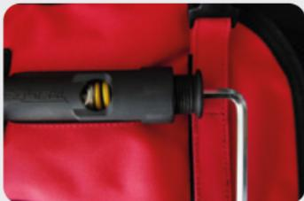
Loosen the bearing cap using the Allen key (5 mm) supplied with the airbag. Do not unscrew it fully but just enough to put the piston back in place.
